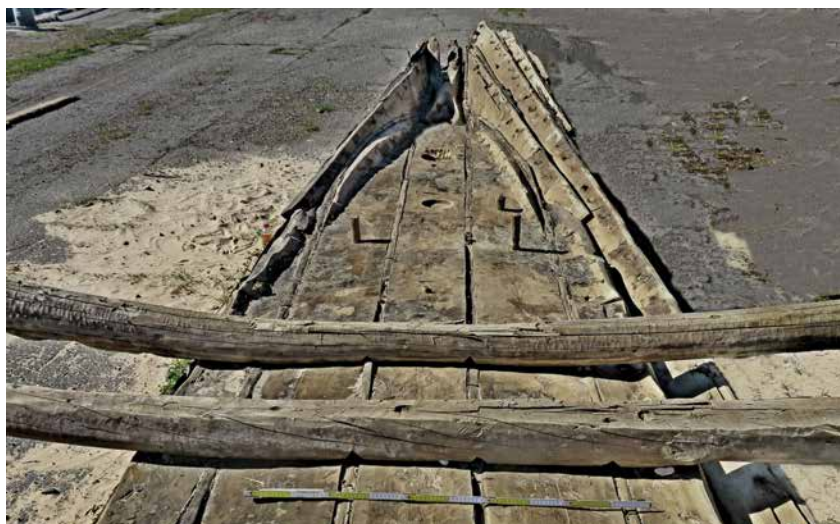
Fig. 4 The bow tip of the vessel: the connection of the starboard side to the stem (photo: P. Sorokin)
