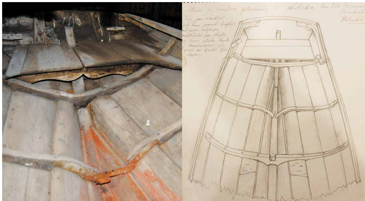
Fig. 2 The spiral-grown and hand-hewed plank called karmvinda. The author's photo of the original boat is on the left, and a sketch from the Nordic Museum is on the right (photo: F. Leijonhufvud; Nordic Museum archives).
