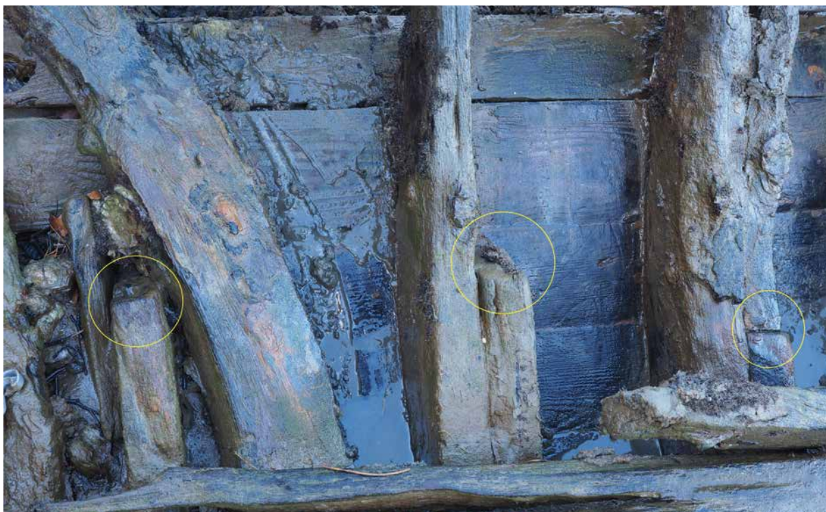
Fig. 2 Details of the floor frame head and futtock heel on the Mendexa I double frames. The futtock for the middle and left frames is not present but the floor frame head can be seen cut and ready to join the futtock. This joint can be seen on the right floor frame and futtock (photo: J. M. Matés Luque).
