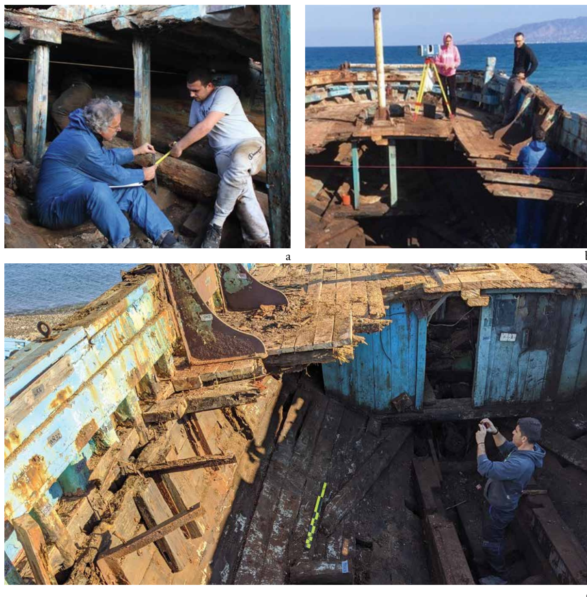
Fig. 3 The different methods of recording Agios Spyridon: a) Conventional measurements, b) Laser Scanning, and c) Photogrammetry
