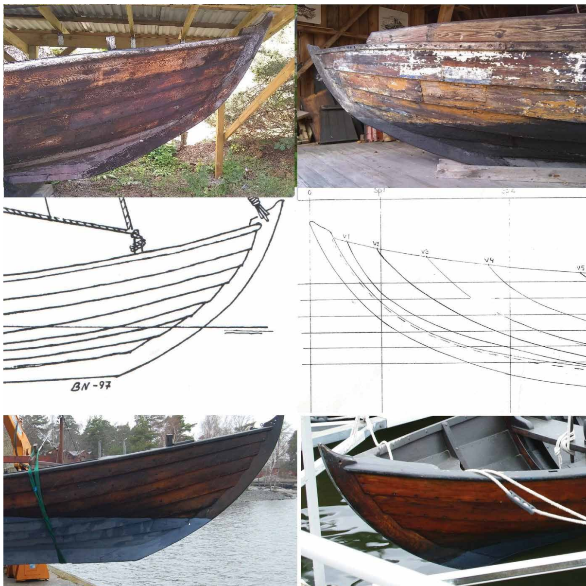
Fig. 4 Stem shape of original boats interpreted with the characteristic shape smoothened out by the replica builders (photo: F. Leijonhufvud).
