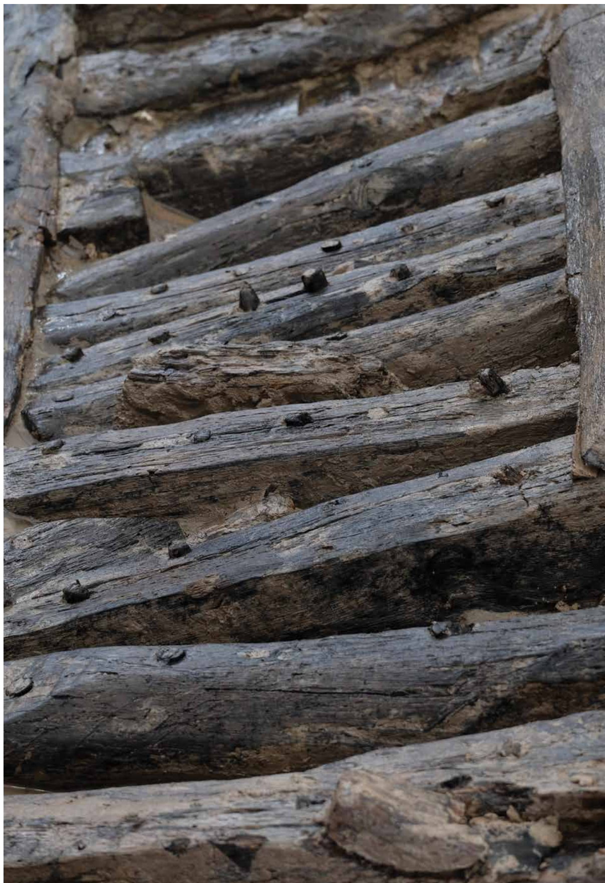
Fig. 6 Detail of the treenails in the starboard frame (photo: P. Ernaux, Inrap)
